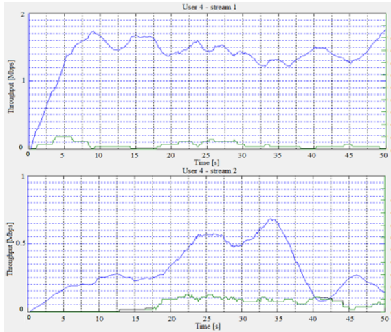
Figure 4. Exp.1 - Throughput and BLER for User 4 when PF scheduler is used
