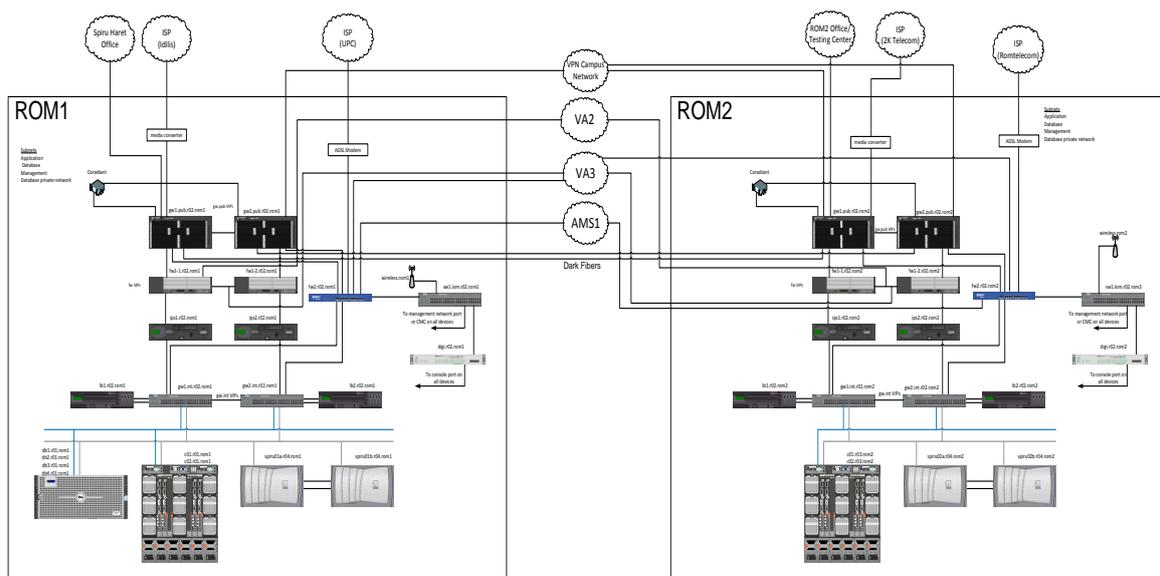
**Figure 5.** Hardware architecture of an e-Learning system and a disaster recovery plan (DRP) implemented
