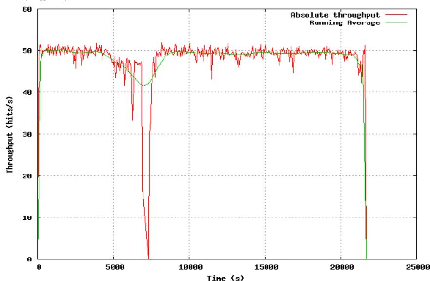
**Figure 4.** The graph resulting from the test on stability when loading over the designed limit and recovery without intervention after a simulated failure.
