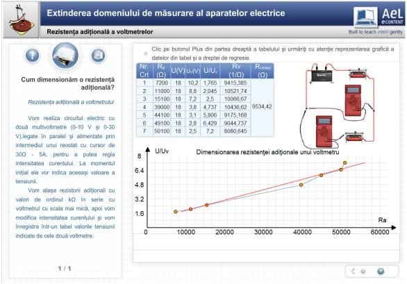
Figure 3. The additional resistance of voltmeters [6]
