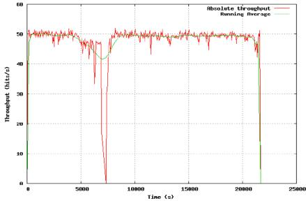
**Figure 4.** The graph resulting from the test on stability when loading over the designed limit and recovery without intervention after a simulated failure.
