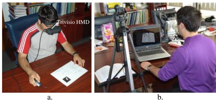
**Figure 1.** The Trivisio see-through AR HMD (a) and the Desktop AR system (b)
