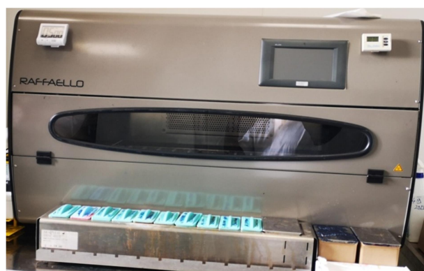
Fig. 8. Colorarea – autostainer liniar („robot stainer”) – 10 programe simultane, capacitate ~250 lame/ zi
